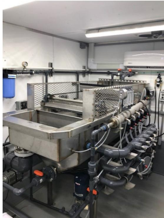
**NClear's pilot trailer, with custom-built DAF, chemical feed tanks, floc tubes.**
